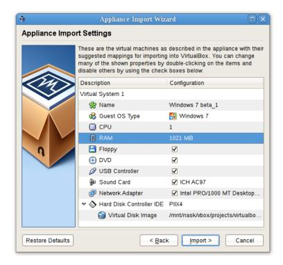
This presents the virtual machines described in the OVF file and allows you to change the virtual machine settings by double-clicking on the description items. Once you click on "Import", VirtualBox will copy the disk images and create local virtual machines with the settings described in the dialog. These will then show up in the list of virtual machines.
